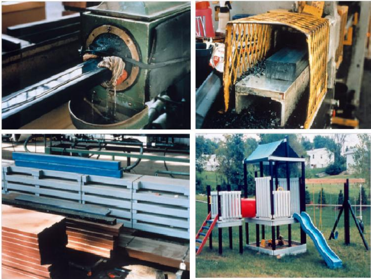
Figure 4. Recycling of HDPE into plastic lumber
